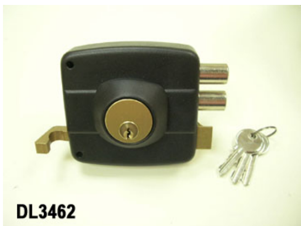
DL3462 Steel Drawback Lock with Brass Latch & 2 Steel Cylindrical Bolts, Brass Internal Cylinder & Half Brass External Fixed Cylinder with Steel Cylinder Cover, 3 Brass Keys, 2 Throw, Paint Finished, Size: 100mm
